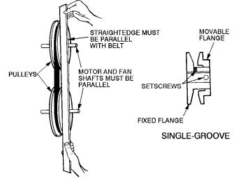
Fig. 19 — Indoor-Fan Pulley Adjustment
